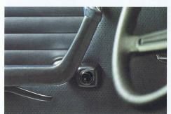
Wing mirror adjuster. Control lever in a protected position on the inside of the driver's door.
