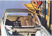
Checking the strength of the roof pillars and roll-over bar if the car overturns.
