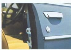
.BMW door lock with ball catch and safety anti-burst strikers - do not open on impact.
