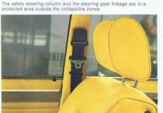
Systematic safety thanks to the standard combination of head restraints (angle adjustable) and inertia reel seat belts.
