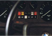
Automatic transmission indicator strip showing position of selector lever (standard on BMW 3.3 Li. otherwise as optional extra)
